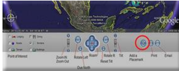
Figure 9: Google Earth Control Panel (Add Placemark Tool Circled in Red on the Right)
